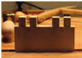
Wasted away. This is the result after clearing the waste between the tenons by sawing close with a bow saw then cleaning up with chisels – using the shoulder line as a guide.
